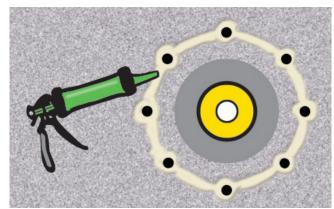
3. Apply **sealing compound** material on the wall with a hand pistole circular around every screw bore as well as the complete core bore range.
