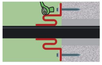
5. Push the side of the Compenseal® with flange bore holes first over the media pipe, collar facing the wall. After that interlock Compenseal® with pressure plate and **spread** emergent **sealing compound**.
