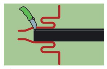
4. If necessary, cut down the seals nozzle to the correct pipe dimension.
