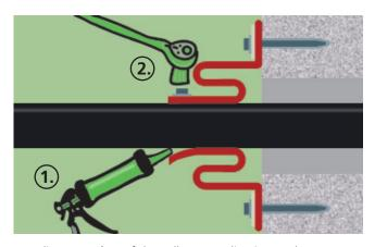
Adjust opening of the collar to media pipe so that a wave shaped expansion zone occurs. Inject sealing compound circularly into the collar opening and fasten strap tightly afterwards.
