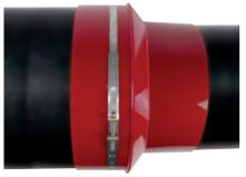
2. Fit the supplied steel-strap with max. 10 Nm at the front end of the sleeve on the casing pipe
