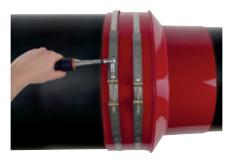
Fix second strap with max. 10 Nm (smoothen escaping sealant).
